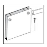
Nylon bushes with screw fixings secure directly into the wall studs
